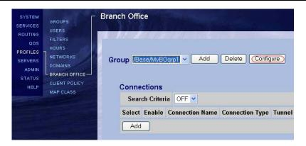
The selected BO group's current configuration page will appear. As shown in the figure below, the NVR's IKE and IPSec settings do not completely match with the Secure Router so we have to modify the NVR's configuration to match the SR. To do this, click on the IPSec Configure button.
