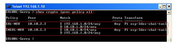
**Note:** At this stage, Branch Office Tunnel can be established as long as traffic is initiated from the SR side (assuming NVR has been configured already). If you want traffic to be initiated from the NVR side, then the SR must be manually configured to accept IKE negotiations which will be discussed on the next step.
