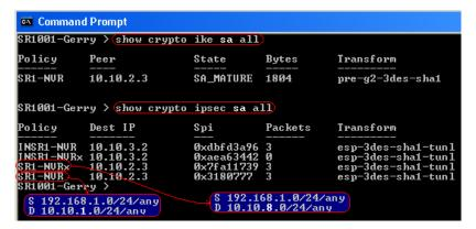
In NVR, as shown in the figure below, you should be able to see one BO session with two connected subnets. Click on the 'Details' button and you should see 10.10.1.0 - 192.168.1.0 and 10.10.8.0 - 192.168.1.0 connected subnets.
