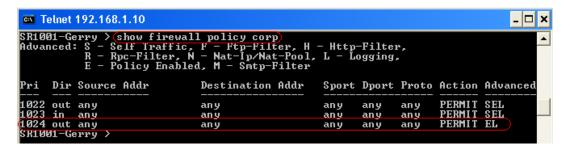
As such, the SR must be manually configured to allow *inbound* transit traffic from a particular source network (this will be 10.10.1.0/24 in our example) to a particular destination network (this will be 192.168.1.0/24 in our example). To do this, edit Firewall policy *Corp* and then type 'policy <pri>cpriority/rule number> in address 10.10.1.0 24 192.168.1.0 24'. To see the added policy for Firewall policy Corp, use the CLI command 'show firewall policy corp'.
