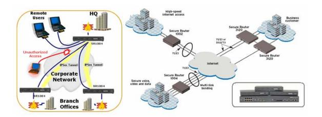
As of today, the Nortel Secure Router platform consists of SR 100x series and SR 3120. The SR 100x series are ideal for installation in small to medium enterprise remote sites and branch offices while the SR 3120 platform is ideal for medium to large branch and regional enterprise environments.
