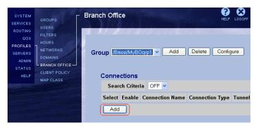
Under Add Connection page, enter your preferred BO connection name. Ensure that tunnel type is IPSec and connection type is Peer-to-Peer. Click on the OK button.
