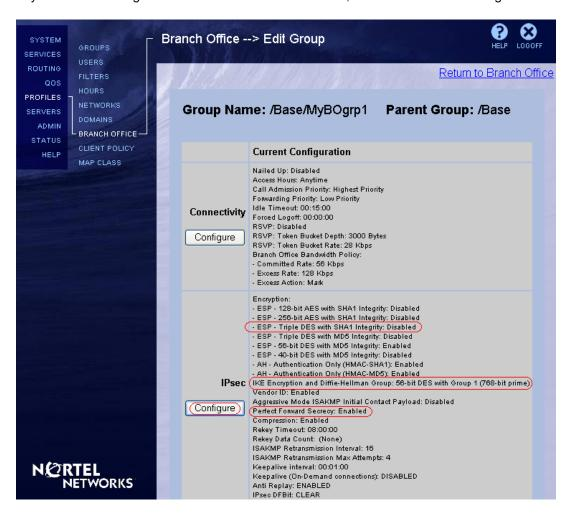
The Secure Router is configured for one IPSec transform proposal which is ESP – 3DES – SHA1 so we must configure the same proposal on the VPN Router to have a match in order to successfully establish the VPN connection. Under encryption field, enable ESP – Triple DES with SHA1 Integrity.
