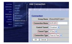
Under BO connection configuration page, check/select Enable to enable the connection. Then select the Local IP address (this would be 10.10.2.3 in our example) as the local endpoint and enter the Remote IP address (this will be the IP address of the Secure Router which is 10.10.3.2 in our example) as the remote end point or the peer address. Under authentication, select Text Pre-Shared Key and enter the secret key. The secret key must match with the secret key configured on the Secure Router.
