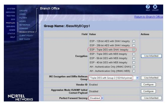
**Note:** If the desired IPSec transform proposal (shown on the right side of the encryption field) and/or the IKE encryption & DH group is/are not listed in the available options, go to Services > IPSec page and enable/check the desired IPSec transform (shown under encryption portion) as well as the desired IKE encryption and DH group.
