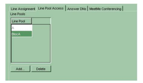
For sets that need access to the SIP trunk they must have access to BlocA (or the Bloc that the SIP trunks are assigned to).
