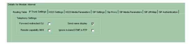
Forward redirection OLI: off Remote Capacity MWI: off Send name display: on Ignore in-band DTMF in RTP: off
