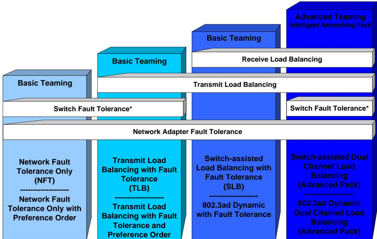
\* Switch Fault Tolerance means Team supports members connected to more than one switch.
