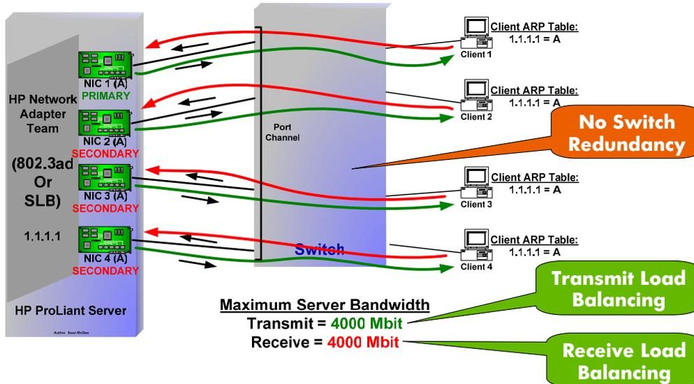
Dual Channel and Dynamic Dual Channel were developed to address the predicament of having to choose inbound load balancing (SLB or 802.3ad) versus switch redundancy (NFT or TLB). With Dual Channel, a server can have full transmit and receive load balancing with switch redundancy (refer to Figure 4-20).
