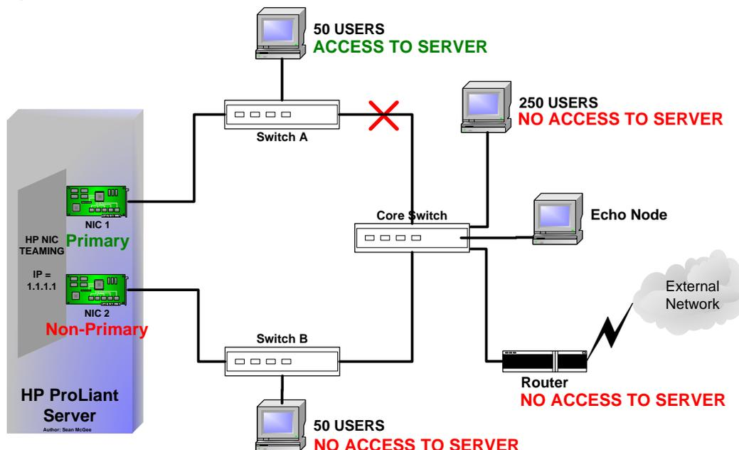
To solve this problem, HP Engineering developed the Active Path mechanism. The Active Path mechanism allows the teaming driver to actively monitor network connectivity on a per-team member port basis with an external network device (designated as the Echo Node). Team member ports that have connectivity with the Echo Node
