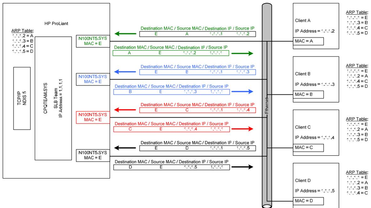
Unlike NFT and TLB, SLB does not utilize the concepts of Primary and Non-Primary ports within a team. All ports within a team are considered equal and perform identical functions as long as the particular port is in a functioning state. The algorithm for load-balancing transmit traffic used by SLB is identical to the algorithm used by TLB. Unlike TLB, SLB load balances all traffic regardless of the protocol being used.
