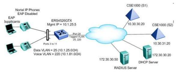
In the 5.1 software release for the ERS4500 and ERS5500, non-EAP support for Nortel IP phones was introduced. This feature allows a Nortel IP Phone and an EAP Supplicant to co-exist on an EAP enabled port. The IP Phone will not require authentication while the device attached to the IP phone will have to be authenticated via EAP.
