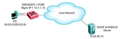
Assuming we wish to provide RADIUS authentication using the non-EAP clients MAC addresses password via port 9 of ERS4550T-1-PWR, please follow the following configuration steps.
