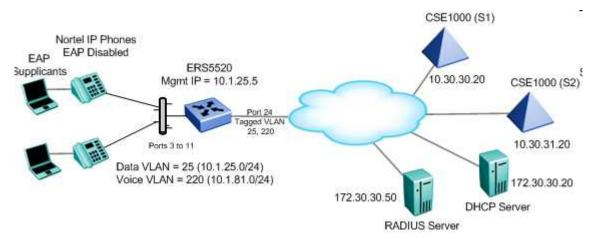
For this example, we will demonstrate how to configure the Ethernet Routing Switch 5500 to allow for non-EAP (NEAP) authentication via RADIUS for the IP Phones. We will also demonstrate using user based policies to apply QoS for the IP Phones. Hence, instead of configuring filters on the switch to apply QoS for the voice traffic, we can use a policy triggered by EAP to apply QoS to the voice VLAN.
