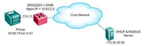
Assuming we wish to provide RADIUS authentication using the non-EAP clients MAC addresses via port 1/9 of the ERS2526T-1-PWR stack. In this example, we will assume the NEAP client will not be mobile, i.e. a printer, such that it has a static IP address and is permanently connected to port 1/9. This will allow us to use a NEAP password consisting of the client MAC address, IP address, and switch port number.
