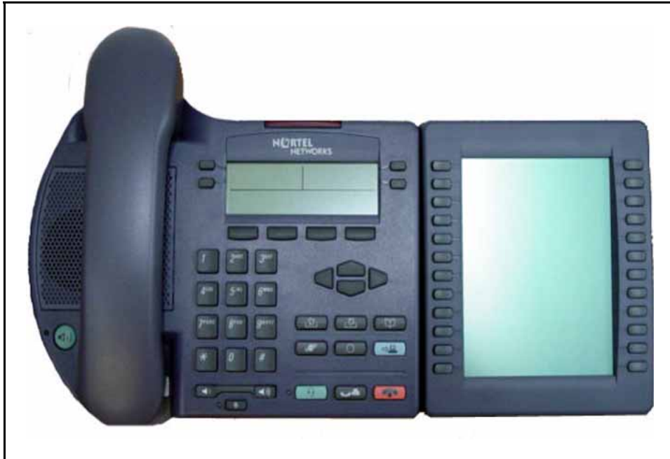
Figure 10 IP Phone 2002 with one IP Phone KEM attached
